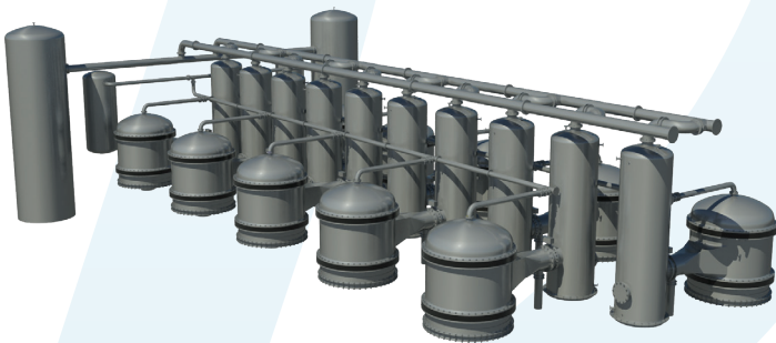
Design of a 120 MLD full-scale CeraMac plant.
